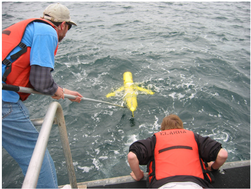
OSU researchers recover an underwater glider from the stern of OSU's coastal research vessel the R/V Elakha . Photo by Jack Barth, OSU.
