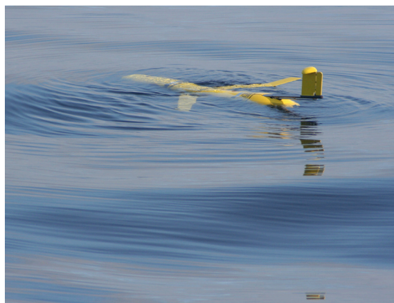
Autonomous underwater glider operated by Oregon State University capable of measuring physical and biological properties of the upper ocean. Changes in buoyancy make the glider move up and down while the wings allow the vehicle to move forward. Satellite cell phone and GPS antennae are contained in the tail fin. Photo by Susan Holmes (OSU).
