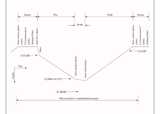
Figure 1. A schematic of a Seaglider autonomous run profile, with run phases indicated by the intervals at the top of the figure and the profile data boundaries indicated by the interval at the bottom of the figure. The figure is not to scale in either dimension.
